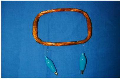
Fig.4 Prototype of Magnetic Torquer
