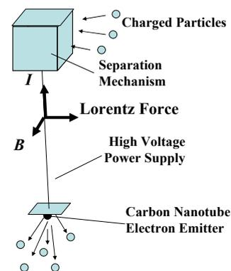
Fig.5 Tether Deorbit System
