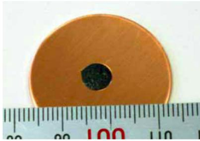
Fig.6 Prototype of Carbon-nano-tube Emitter
