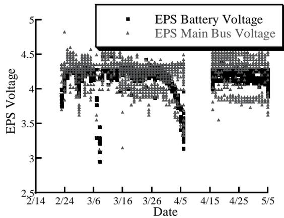
Fig. 6 Flight Data of Battery and Main Bus Voltages
