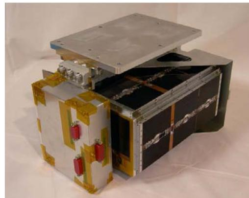
Fig. 5 Cute-1.7 + APD#1 and the Separation System
