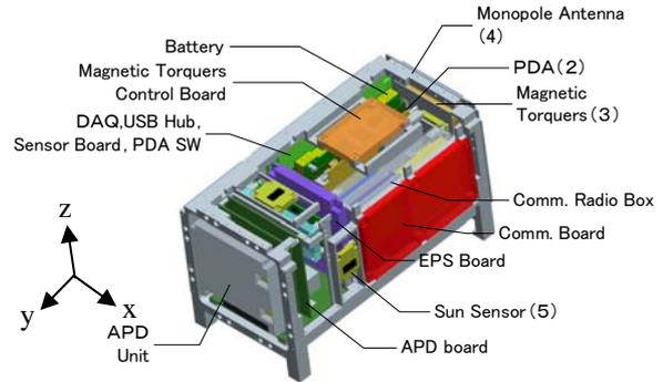
Fig.3 Components layout
