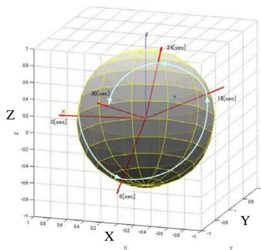
Fig. 9 Direction of the sun in body fixed coordinate system
