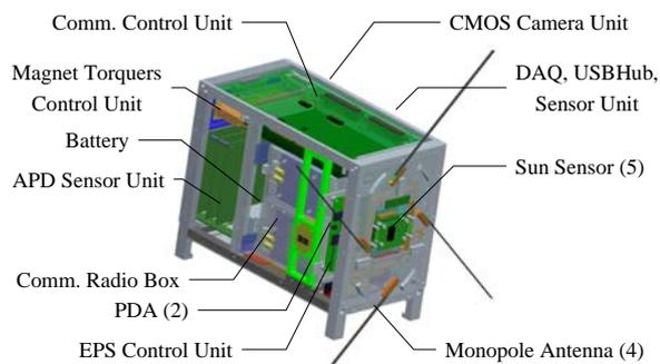
Fig. 10 Cute-1.7 + APD#2 Components Layout
